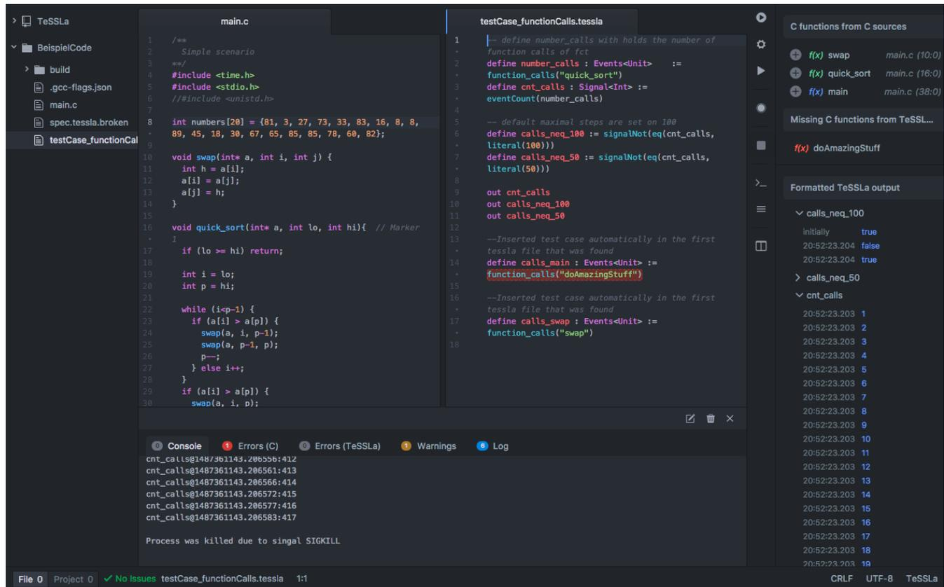
Figure 3: Atom plugin for TeSSLa based runtime verification of C programs.
