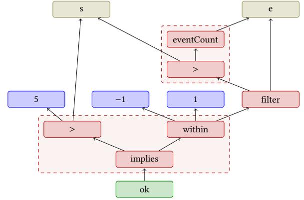
**Figure 1: The dependency graph for the spec in Example 2.1. Inputs are shown in brown, constants in blue, outputs in green, computation nodes in red and some possible merges of computation nodes in dashed red.**
